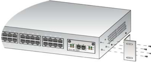
Figure 4.2a Secure brackets onto Compex SXP2224WM
